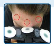
3. Pull the black headband over your head. Press firmly on the outer edges of all three sensors to ensure complete contact with your forehead.
