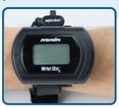
2. Place your finger fully into the gray sensor with the cable facing up. The wrist device will turn on automatically.
